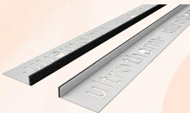
Ultratherm® insulated plastic trim beads for use around window and door frames to reduce cold bridging. Also allow windows and doors to be replaced without damaging the insulation system.
